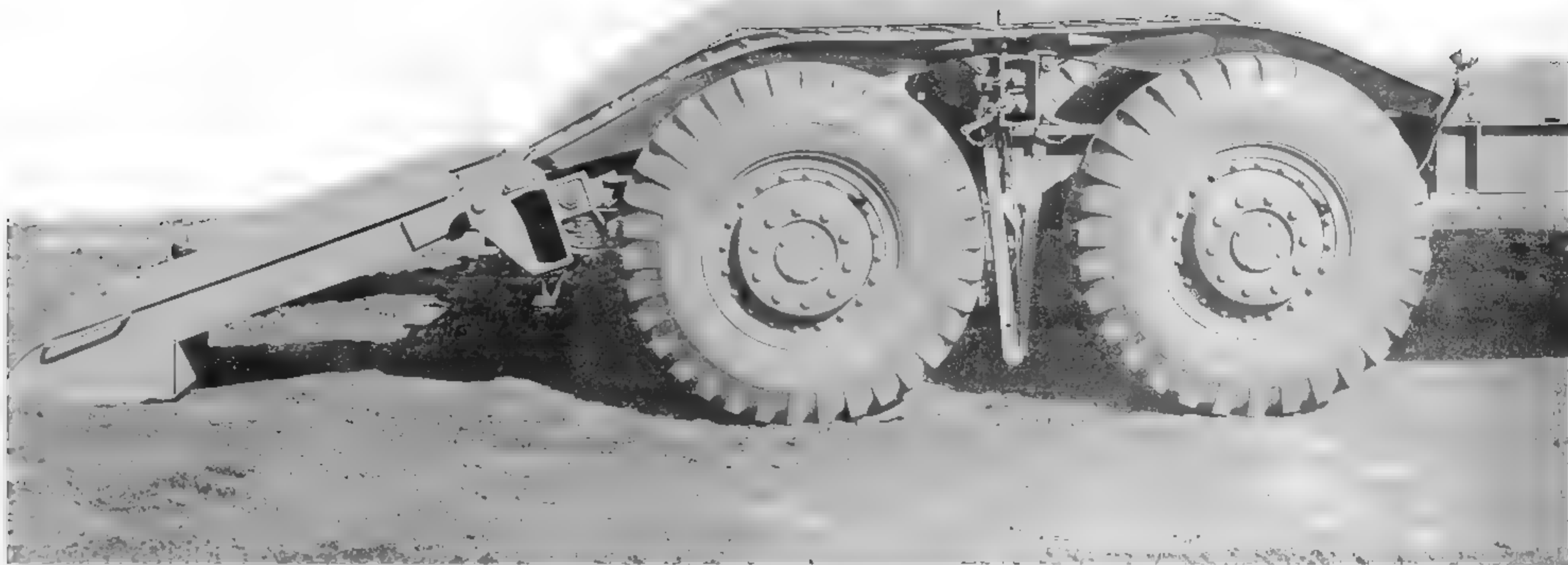
In this view the M15 wheel covers have been lowered, as have the ramps, into the loading position. (U.S. Army photo)
